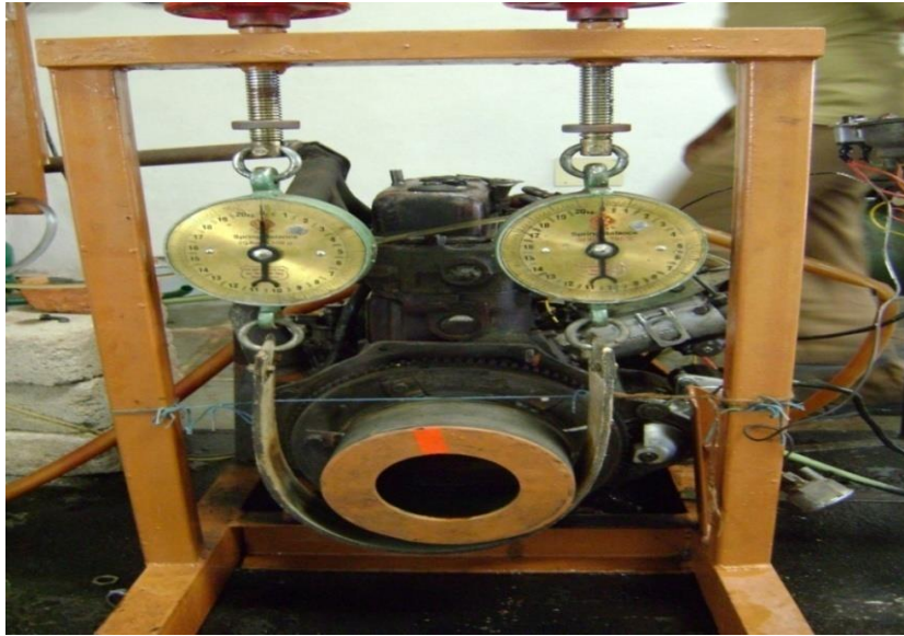
Fig.2 Experimental loading set up of 20 hp diesel engine with mechanical loading With turbocharger
